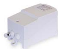
H15 In-line two-position valve R1/2", for 2-pipe systems. The valve is operated with an electric thermal actuator (ON/OFF, 24 Vac).
