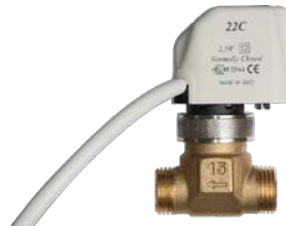
H25 In-line two-position valve R1/2", allowing easy connection to a 2-pipe system. The valve is operated with an electric-thermal actuator (ON/OFF control, 230 Vac).
